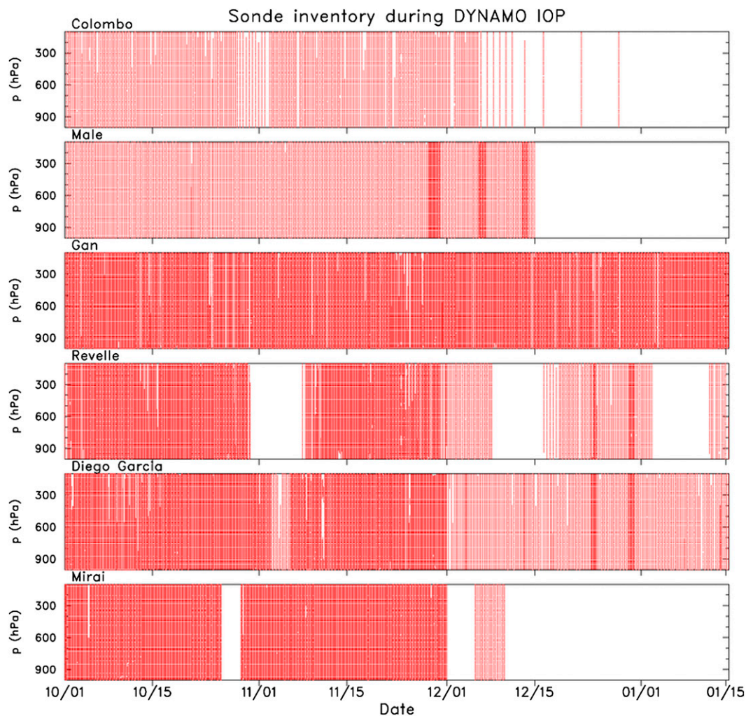
FIG. 2. Visual sounding inventory of upper-air data for six core sites based on L4 data (i.e., 5-hPa interpolated). Each line of dots represents a successful sonde launch. Larger data gaps at Revelle and Mirai are the result of ship port calls.
