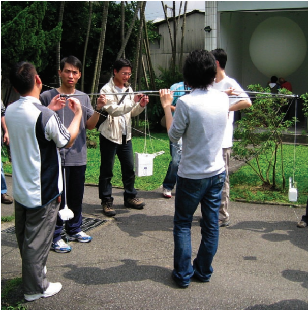
FIG. 4. Taiwanese scientists prepare for an intercomparison sonde launch in Banchiao, Taiwan, on 15 Apr 2008. In this launch, a trirod structure was utilized to compare three sonde types (Meisei, Graw, and Vaisala RS92).
